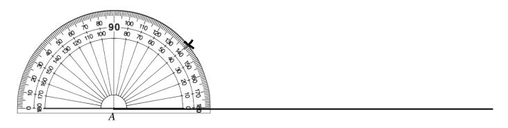
Step 2: Draw side c, which is 8 cm long. Label the end of the line B.
