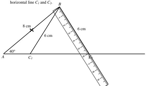
We have constructed two triangles which satisfy  $A = 40^{\circ}$ , a = 6 cm and c = 8 cm.
