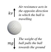
As the velocity v of an object increases so does the air resistance acting on it. Let  $F_r = kv$  for some constant k.
