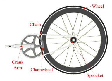
Suppose the length of the crank arm is  $r_1$  and the rider exerts a force on the pedal of  $F_p$ .
